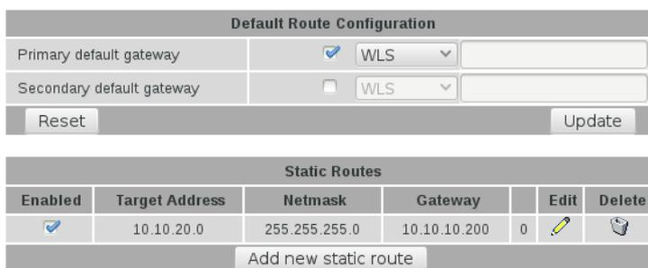
Figure 169: Static route table with route 2 removed
