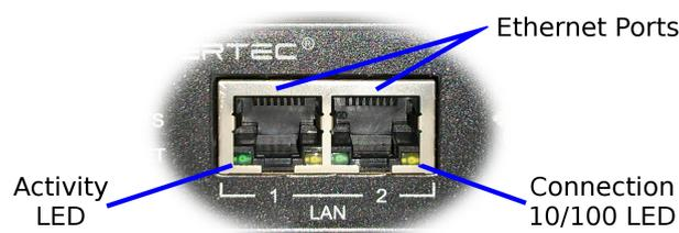
Figure 6: Ethernet ports.
