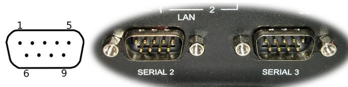
Figure 8: DTE Serial ports.
