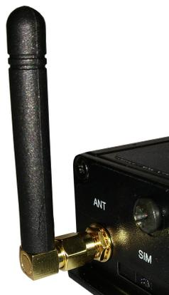
Figure 14: Antenna connected to SMA connector.
