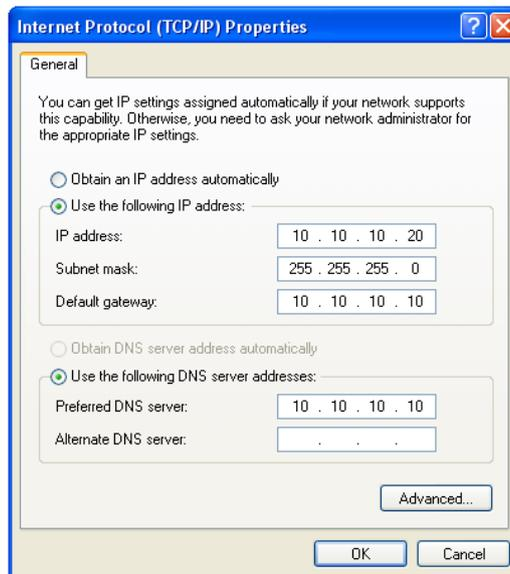
Figure 18: Internet Protocol (TCP/IP) Properties dialog box showing the recommended IP settings.
