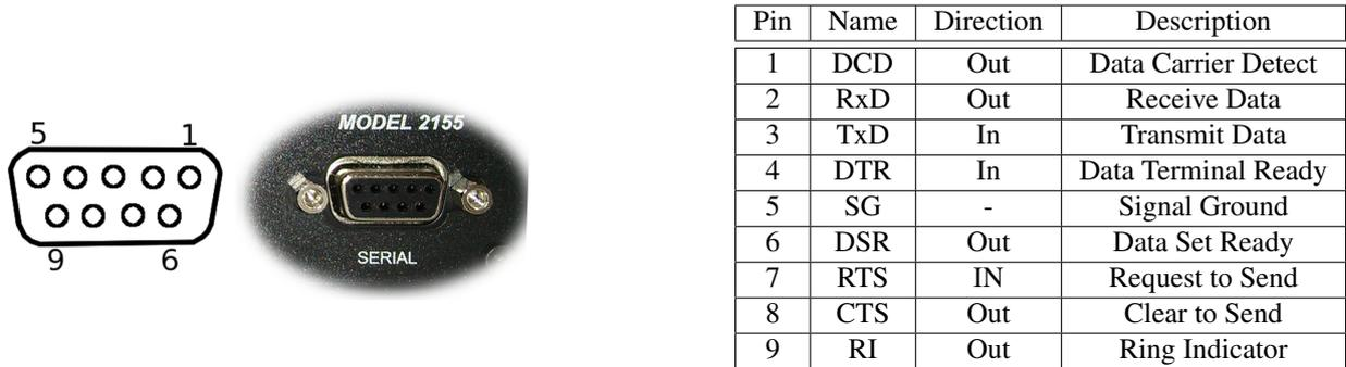
Figure 7: Modem / DCE Serial port connections.
