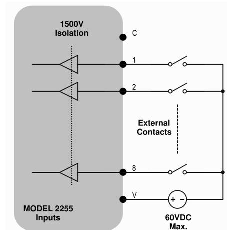
(b) Digital Input wiring with external voltage source.
