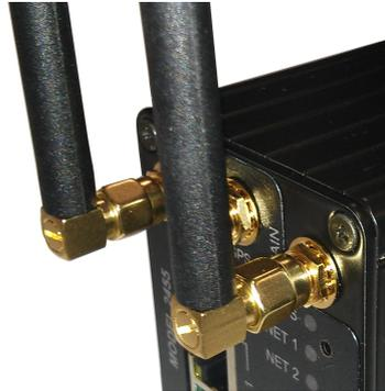
Figure 6: Antenna connected to SMA connector.
