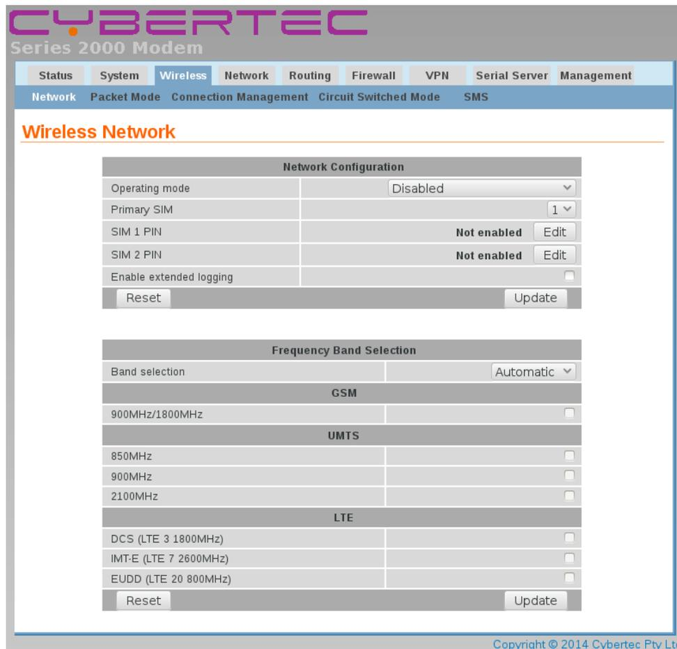
Figure 12: Wireless Network configuration.
