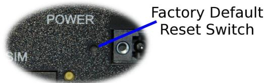
Figure 11: Factory Default Switch access.
