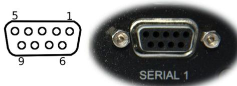
Figure 7: Modem / DCE Serial port.
