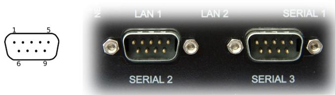
Figure 8: DTE Serial ports.
