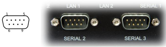
Figure 8: DTE Serial ports.
