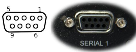
Figure 7: Modem / DCE Serial port.
