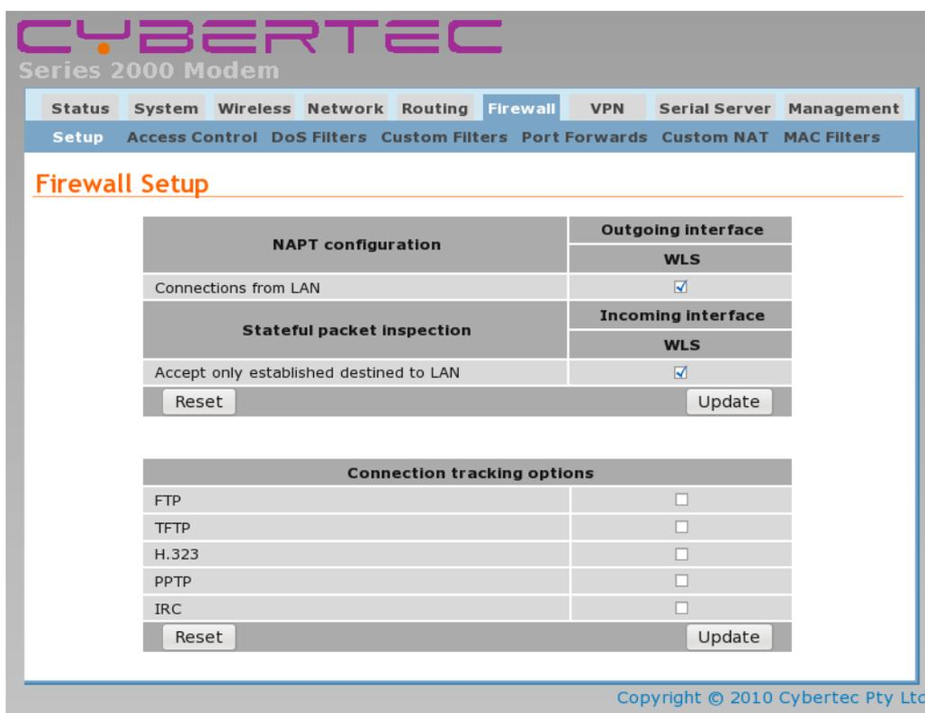
Figure 152: Basic firewall configuration
