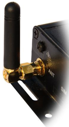
Figure 15: Antenna connected to SMA connector.
