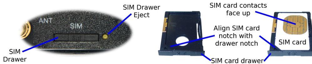
Figure 14: SIM card eject button.
