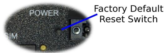
Figure 11: Factory Default Switch access.
