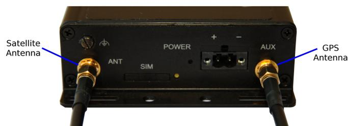
Figure 19: Antenna cables connected to SMA connectors.
