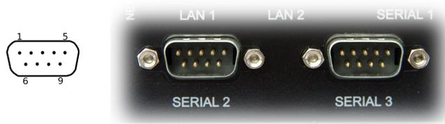
Figure 8: DTE Serial ports.
