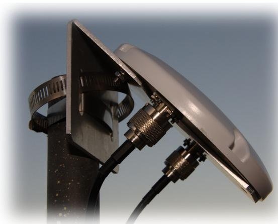
Figure 15: Fixing the antenna to the bracket.
